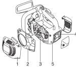
Clean the cooling system with a brush once a week, more often in demanding conditions. A dirty or blocked cooling system results in the machine overheating which causes damage to the piston and cylinder.
